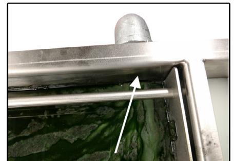
Fluid level in raised position in order for tramp oil to exit the separator
