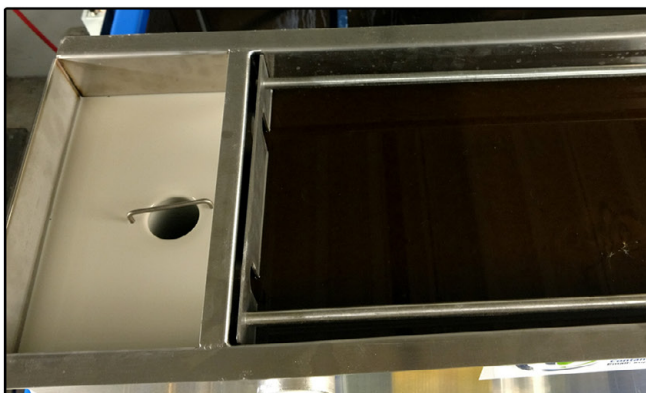
Buildup of Tramp Oil in CrossFlow and CF20 Separators
