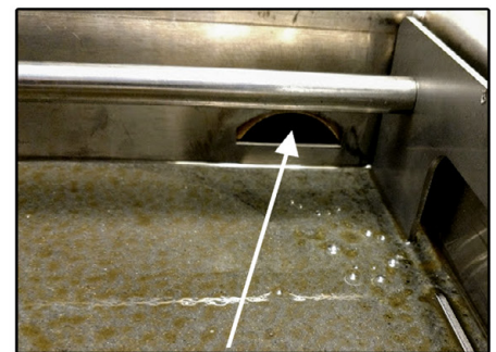
Fluid below the half-moon tramp oil discharge prior to fluid level being raised
